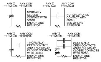
**NOTE:** This option should be selected if either Normally Closed (NC) or Normally Open (NO) detection devices or contacts are being used.
