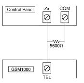
event to the central station. This type of zone always requires a single EOL resistor (5600 $\Omega$ ).
