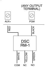
PGM1 can sink up to 300mA of current. Connect the positive side of the LED or buzzer to AUX+, the negative side to PGM1. If more than 300 mA of current are required, a relay must be used. Please study PGM wiring in the accompanying diagram.
