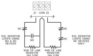
**NOTE:** For UL installations, zone inputs must be terminated with normally closed initiating devices or end of line resistors (1K ohm).
