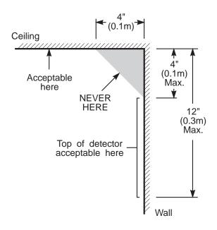
NOTE: Measurements shown are to the closest edge of the detector.
