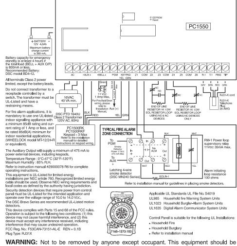
**WARNING:** Not to be removed by anyone except occupant. This equipment should be installed in accordance with Chapter 2 of the National Fire Code ANSI/NFPA 72-1993 (National Fire Protection Association, Batterymarch Park, Quincy MA, 02269). Printed information describing proper installation, operation, testing, maintenance, evacuation planning, and repair service is to be provided with this equipment.
