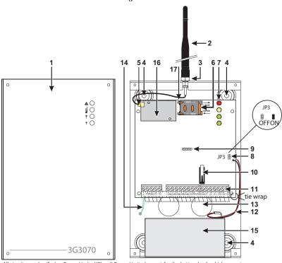
All circuits are classified as Power Limited/Class II Power Limited except for the battery leads which are not power limited. Do not route any wiring over circuit boards. Maintain at least 1" (25.4mm) separation. A minimum 1/4" (6.4mm) of separation must be maintained at all points between Power Limited wiring and all other non-Power Limited wiring. Route wires as indicated above.
