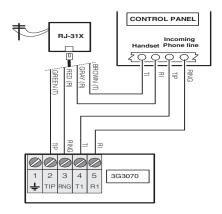
Figure 3 - Power Supply and Supervision Wiring Diagram
