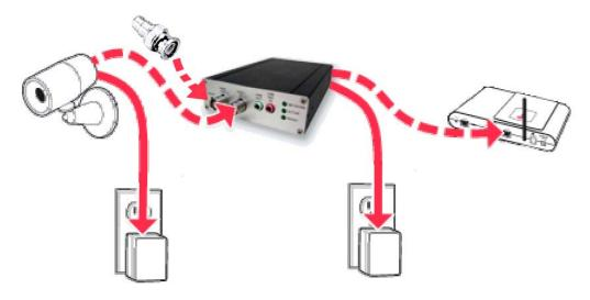
Note: Once connected, the "POWER" and "NETWORK" LEDs on the front of the C24-CAMANL will turn solid green.
