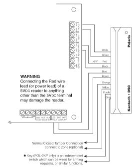
**NOTE**: Only use the +5V power supply when using Polaris Readers.
