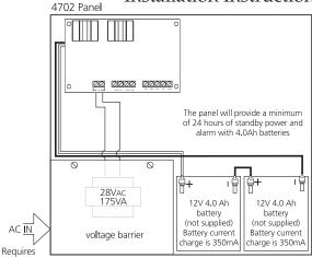
INSTALL BATTERY AND AC WIRING AS SHOWN ABOVE IMPORTANT: A minimum of 1/4" (7mm) separation must be maintained at all points between battery/primary AC/BELL wiring and all other wiring and connections.
